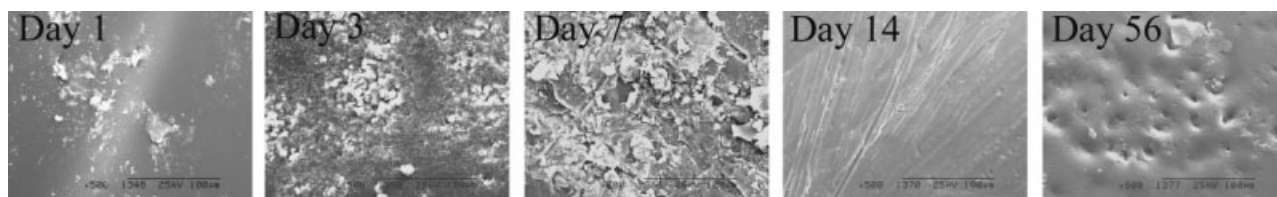
Figure 16 Surface morphology of degraded 70 : 30 PCL-C-DTH/LTP blended films as a function of incubation time as observed by scanning electron microscopy.
